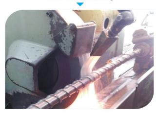
Bimetallic Screw 3rd Process after Nitrading Core Dia Pollishing
